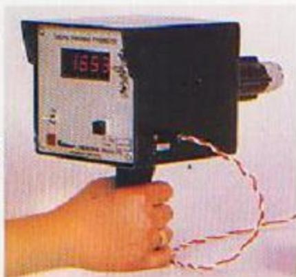
auto battery shut-off are provided as a standard feature. 6/12 mm high, 7 segment, 3 1/2 digit LCD/LED display enables clear visibility. Mains operated battery charger is an essential accessory. **IDEAL**, low cost equipment for foundries.
